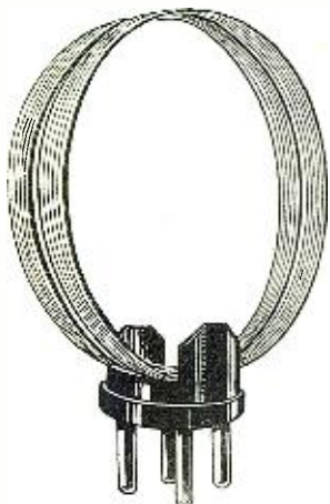
This self-supporting, interchangeable inductance, mounted in a tube base, was awarded second prize.
