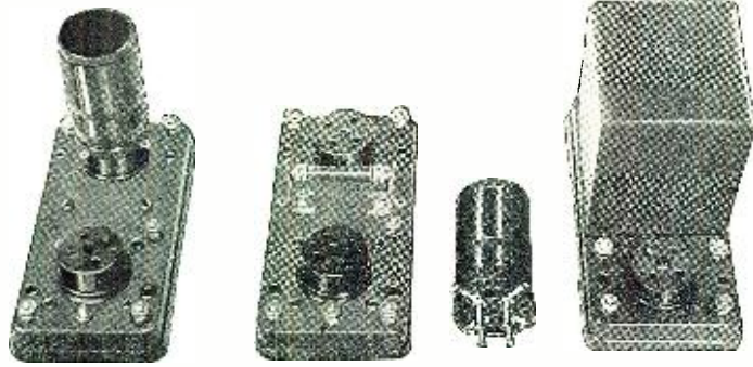
Left: R. F. unit, showing coil in place; center, detector unit, with coil alongside; right, A. F. unit. Each, with the addition of a tube, is a completely self-contained stage of a receiver. Illustrations courtesy Pilot Mfg. Co.
